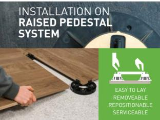
Installation on raised pedestal system exploits the conventional system of floating or raised floors. With this laying system, all the pipes and wiring systems laid beneath the tiled surface can be inspected at any time. It offers instant accessibility, simply by lifting and removing the slabs. Installation on raised pedestal system is used mainly on large, regular surfaces, or above previous floors, provided these show no signs of infiltration.
